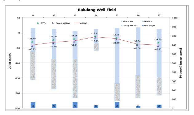
Figure 18 Balulang Well Area – Depth, Screen Location & Discharge
