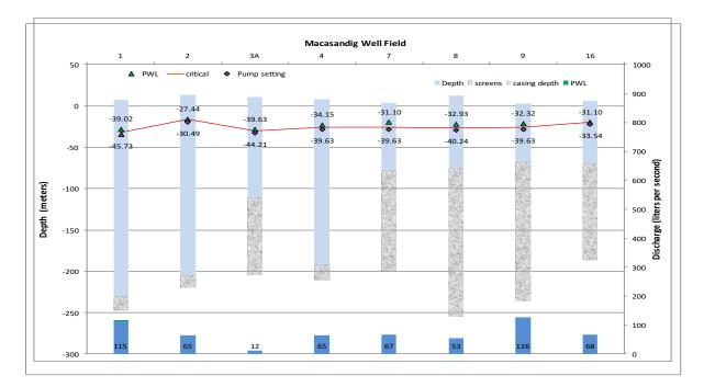
Figure 20 Macasandig Well Area – Depth, Screen Location & Discharge
