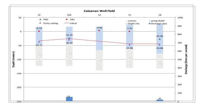
Figure 19 Calaanan Well Area – Depth, Screen Location & Discharge
