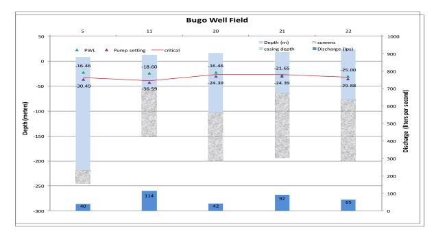
Figure 22 Tablon - Agusan Well Area – Depth, Screen Location & Discharge
