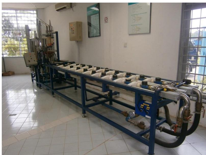
**Photo 50: Semi-Automatic Meter Test Bench (Two Lines with Total Capacity of 10 DN15 Meters)**
