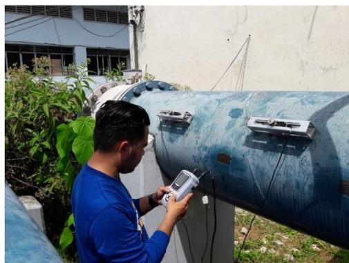
**Photo 45: Actual Installation of Clamp-on Ultrasonic Meter at Macasandig Old Booster Bank #2 Meter**
