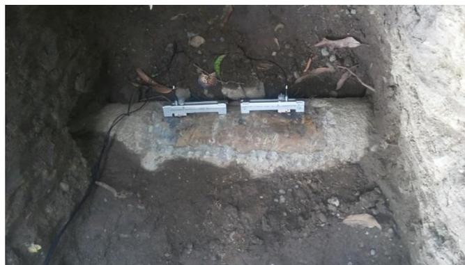
**Photo 42: Actual Installation of Clamp-on Ultrasonic Meter at Bulua Line**
