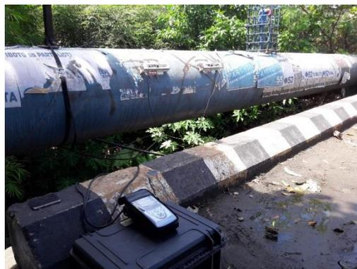
**Photo 43: Actual Installation of Clamp-on Ultrasonic Meter at Bugo Booster Line Meter**
