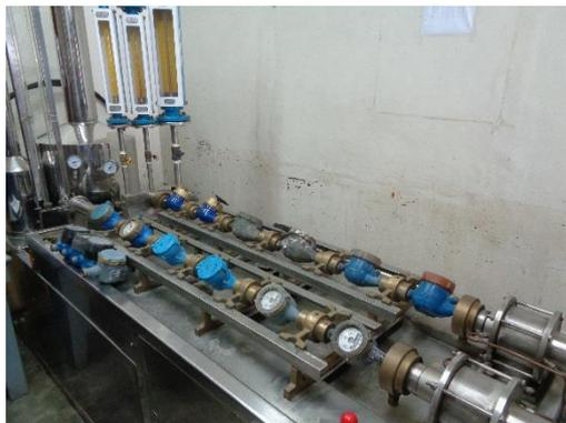
**Photo 24: Meter Error Testing at 45 Degrees Orientation**
