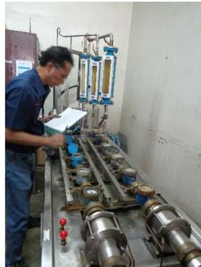
**Photo 23: Meter Error Testing at Horizontal Orientation**
