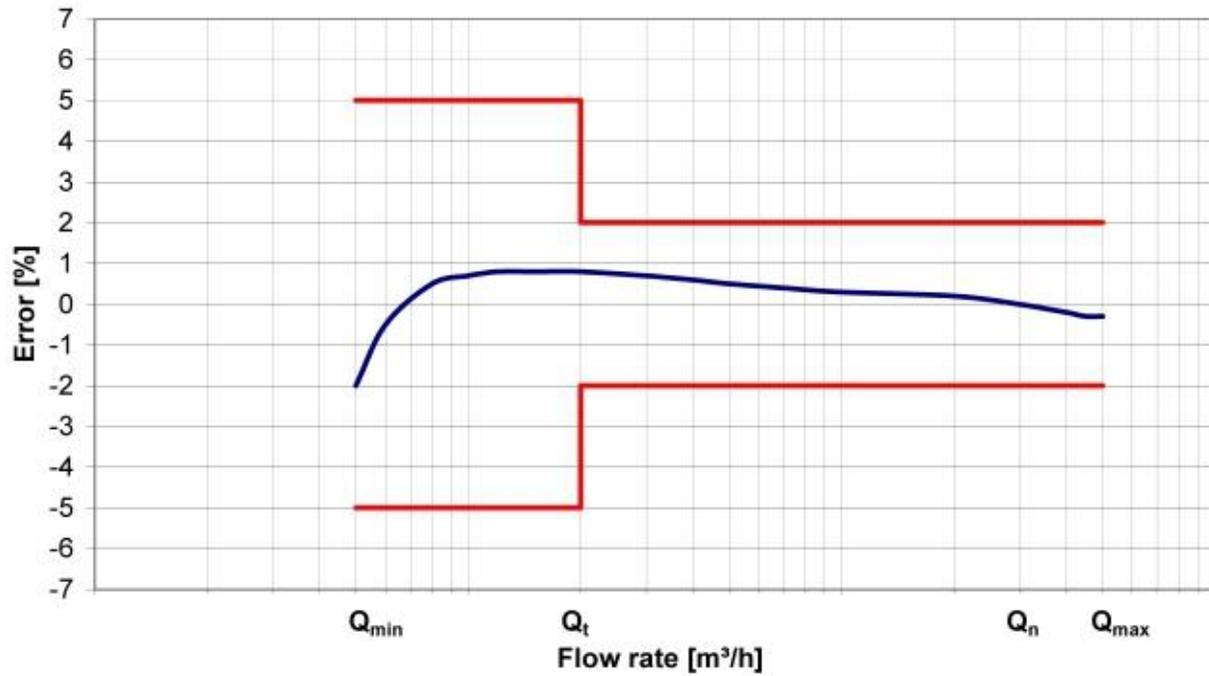
Figure 1: Typical Water Meter Performance Curve
