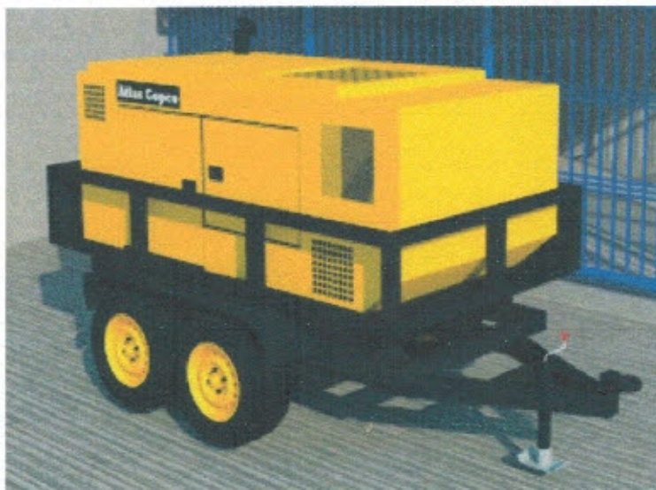
Figure 9 Genset in Mobile Cart
