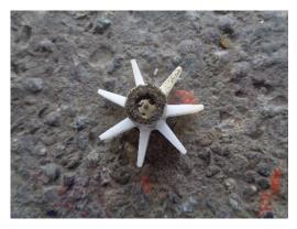
Photo 21: Sand Particles on the Magnet Coupler
