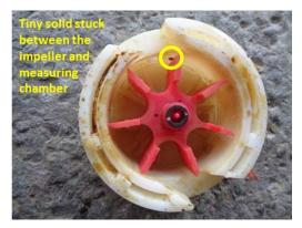
Photo 20: Stuck-up Impeller due to Tiny Solid
