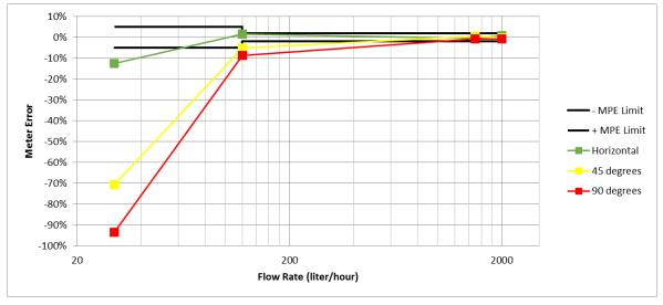
Figure 3: Error Curve of the Water Meter at Different Meter Orientations
