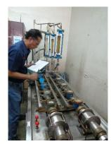
Photo 23: Meter Error Testing at Horizontal Orientation
