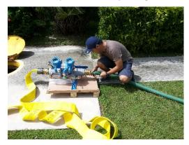
Photo 48: Actual In-situ Meter Accuracy Testing
