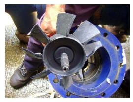
Photo 47: Damaged Turbine of the Large Customer Meter
