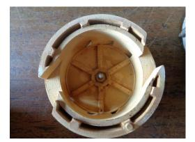
Photo 18: Sediments build-up in the Measuring Chamber
