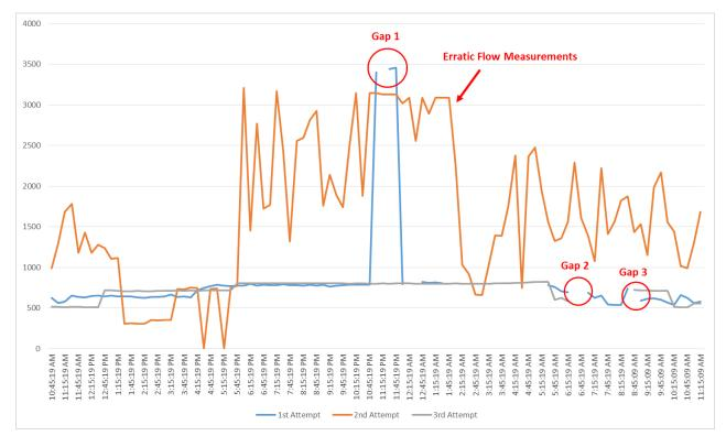
Figure 4: Result of the Three Measurement Attempts in Bulua Line
