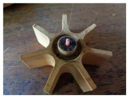
Photo 19: Sediments build-up on the Impeller
