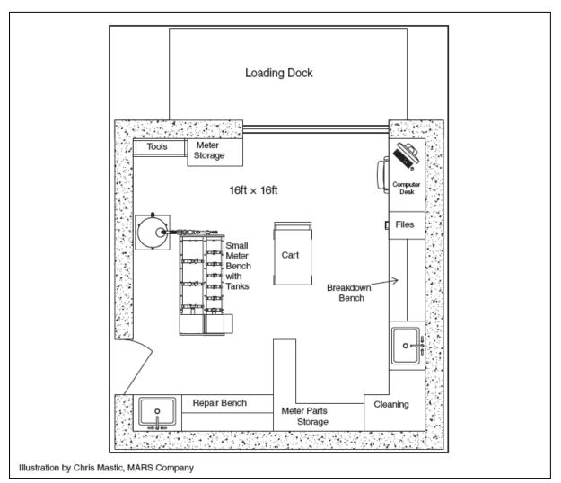
Figure 15: Recommended Meter Testing Facility Workplace for Modern Meter Shop (AWWA M6)
