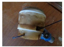
Photo 22: Meter Tampering (Insertion of Plastic Tie)
