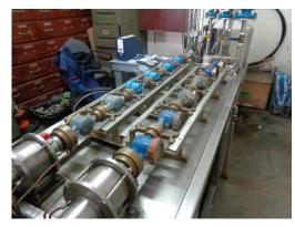
Photo 25: Meter Error Testing at 90 Degrees Orientation
